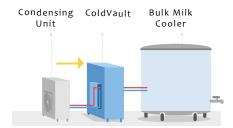
When electricity is available and cooling is not required, condensing unit uses electricity to generate cooling and ColdVault stores it in a phase change material to provide cooling for later use
